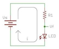
Fig. 8. Current-limiting Resistor Example
