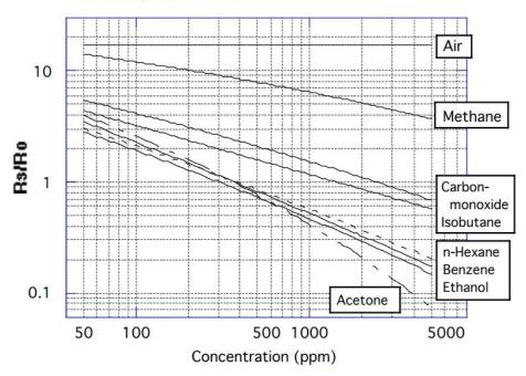
Rs = Sensor resistance of displayed gases at various concentrations
