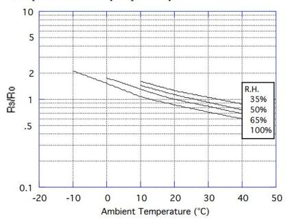
Rs = Sensor resistance at 300 ppm of ethanol at various temperatures/humidities Ro = Sensor resistance at 300 ppm of ethanol at 20°C and 65% R.H.
