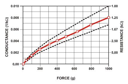
Figure 5.1: Empirical Force-Resistance curve of our chosen FSR
