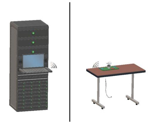
The Physical design above provides a 3-D model of the system. The device itself in this model is located on the table (on the right panel) and is wirelessly transmitting to the server (on the left panel). The speaker for the device will be central to the 4 microphone array. The device will be designed such that it can be placed on any flat surface in a room and be connected to an outlet (not show).
