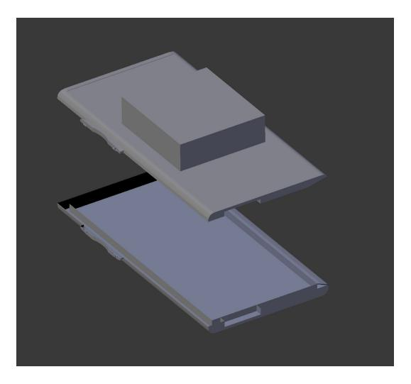
We intend to place the battery pack and the charging module inside the iPod-shaped body, while placing the main PCB in the rectangular extrusion.
