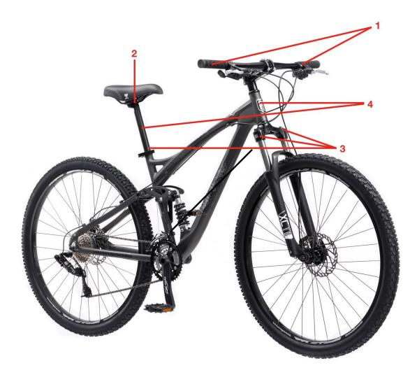
As shown in the figure above, at locations marked "1" on the handle of the bike, LEDs, buzzers and haptic feedback generators will be placed. At location "2", the microcontroller, bluetooth module and power supply will be placed and these will go under the rider's seat. At locations marked "3", the turn indicators/blinkers will be placed and these will be both on the front and back of the bike. Lastly, at locations marked "4", the ultrasonic sensors will be placed.
