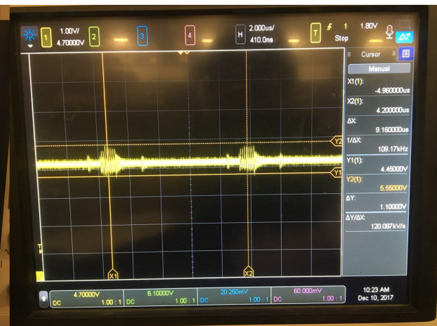
Figure 7: Output 5v voltage with the load
