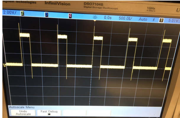
Fig. 20 25% duty cycle using delay method
