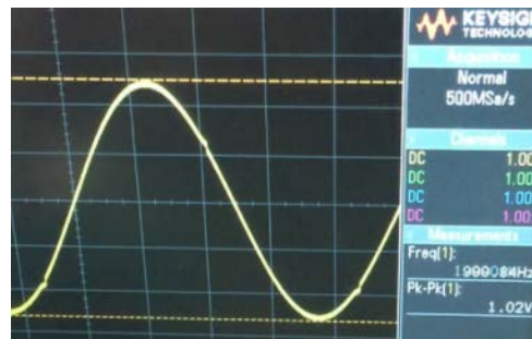
Figure 19. Output of 1.02 V after Unity Gain
