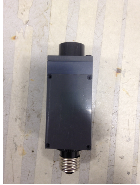
Figure 2: The final, constructed form of the switch box. Figure 3: The final compact form of the light socket device.
