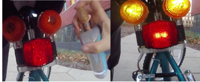
Figure 12: Verification for Brake Light
