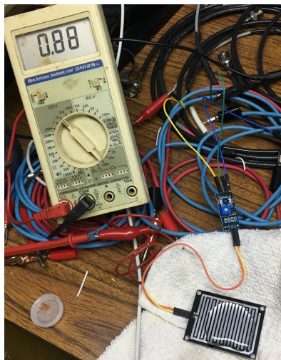
Figure 5: Rain sensor output voltage vs. water coverage
