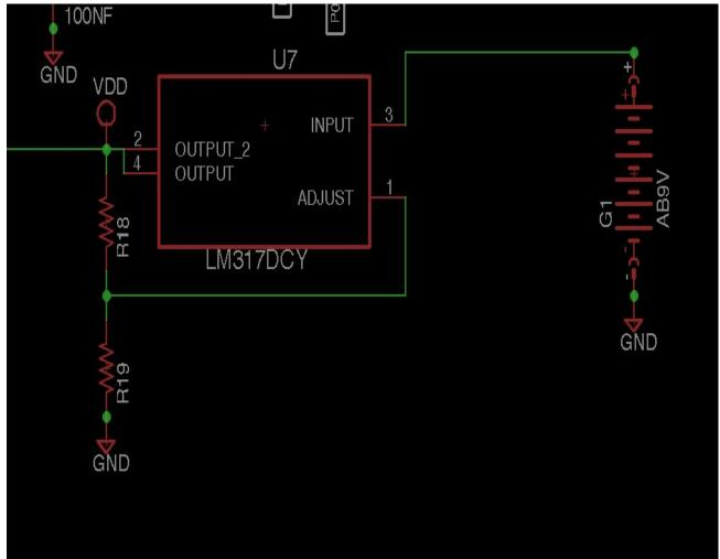
• Simple voltage regulator circuit using LM317 chip.
