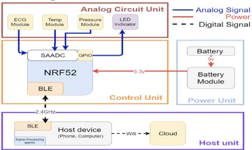
ECG: Electrocardiography SAADC: Successive Approximation A/D Converter GPIO: General-purpose input/output NRF52: Name of our microcontroller BLE: Bluetooth Low Energy
