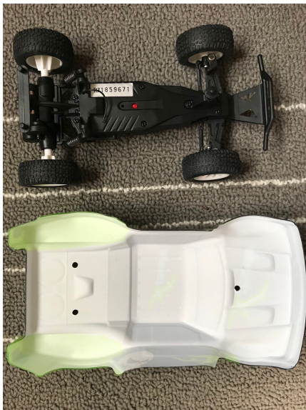
Figures 2-2 (Left) and 2-3 (Right): The Chassis, Body, and Controller of the R/C Car
