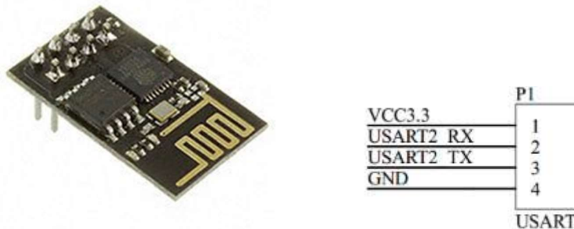
Figure 13 Four Important Pin of ESP8266
