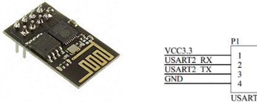
Figure 13 Four Important Pin of ESP8266
