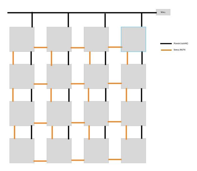
Above is the proposed default topology. Each block is connected to its neighbors via a serial connection and power is distributed via 120VAC rails extending from the wall, into each block and out the otherside, which powers the Pi and LEDs. While other configurations of the system will be supported this will be the default implementation as it most closely matches the space we are going to deploy the system in.
