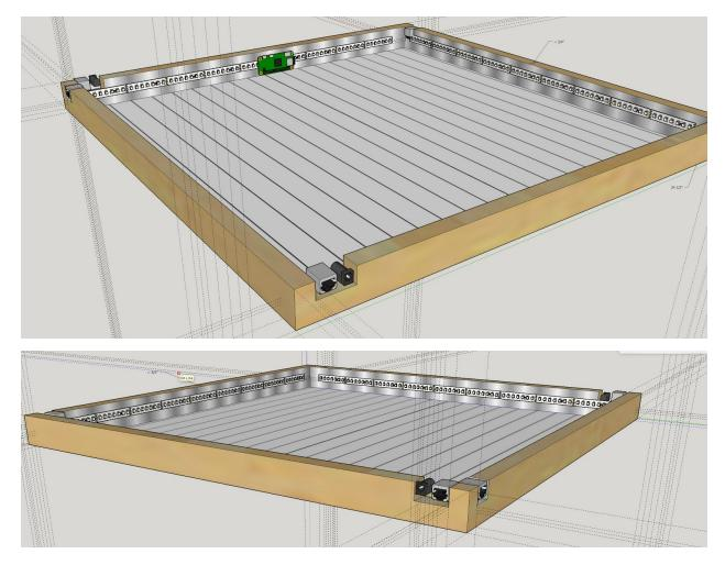
The physical design of the system is as follows; the entire system consists of a collection of units (we are specing to make 15). Each unit is a magnetically suspended wooden box, the same dimensions as a standard ceiling tile (so it is square with external width 24.5" and internal width 23"). On the inside of the box we coat the sides with aluminum tape to reflect the LEDs.
