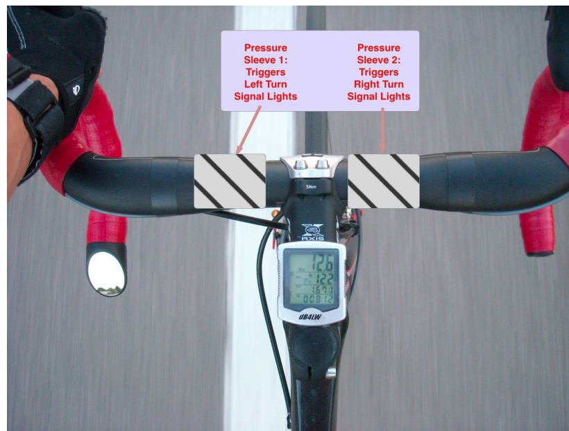
Figure 3. Top-down view handlebars annotated with placement of sensors.
