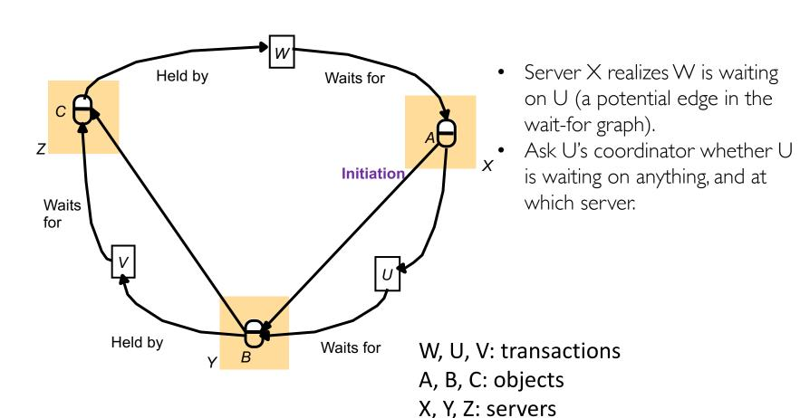
• Edge chasing: Forward "probe" messages to servers in the edges of wait-for graph, pushing the graph forward, until cycle is found.
