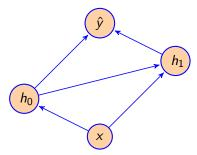
Forward propagation can be summarized by a **flow graph**, which specifies the dependencies among variables, without specifying the functional form of the dependence. For example, the above graph shows that
