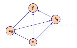
$$\frac{\partial \hat{y}}{\partial h_0}(x, h_0) = \frac{d\hat{y}}{dh_1} \frac{\partial h_1}{\partial h_0}(x, h_0, h_1) + \frac{d\hat{y}}{d\hat{y}} \frac{\partial \hat{y}}{\partial h_0}(x, h_0, h_1)$$
