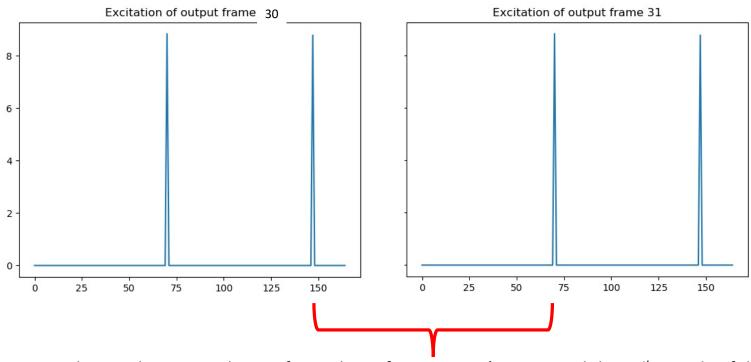
Pitch period = 80 samples ⇒ first pulse in frame 31 can't occur until the 70<sup>th</sup> sample of the frame
