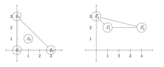
After image warping, the triangle  $\{\vec{x}_1, \vec{x}_2, \vec{x}_3\} = \left\{ \begin{bmatrix} 0\\0 \end{bmatrix}, \begin{bmatrix} 3\\0 \end{bmatrix}, \begin{bmatrix} 0\\3 \end{bmatrix} \right\}$  has moved to  $\{\vec{x}'_1, \vec{x}'_2, \vec{x}'_3\} = \left\{ \begin{bmatrix} 1\\2 \end{bmatrix}, \begin{bmatrix} 4\\2 \end{bmatrix}, \begin{bmatrix} 0\\3 \end{bmatrix} \right\}$ , and  $\vec{x}_0 = \begin{bmatrix} 1\\1 \end{bmatrix}$  is moved to  $\vec{x}'_0$ . Find  $\vec{x}'_0$ .
