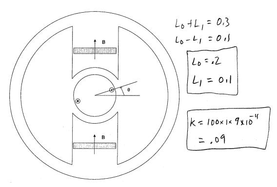
a) Using the general form of the flux linkage given below, find the constants  $L_0$ ,  $L_1$  and K. This flux linkage  $\lambda$  is defined with respect to the voltage labeled as positive where the current enters the page (on the right in the figure) and  $v = d\lambda/dt$ .
