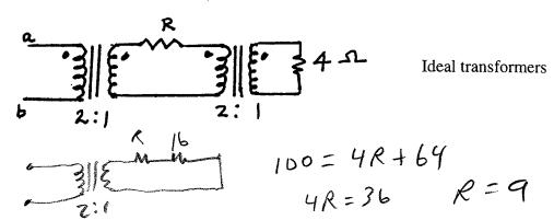
d) Write the two loop equations for the circuit shown
