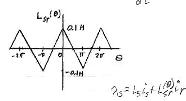
a) Plot the open-circuit stator voltage ( $i_s = 0$ ) as a function of  $\theta$  (label all points)
