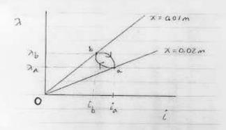
(a) Find the energy stored in the coupling field at point a (use a well-labeled graphical area to give your answer). (Hint: Integration is area under curve)
