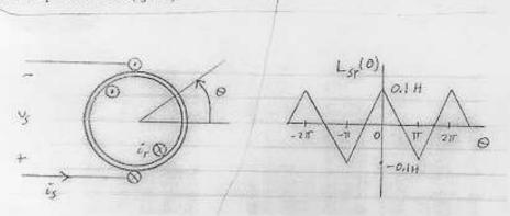
(a) Plot the open circuit voltage as a function of θ (label all points)
