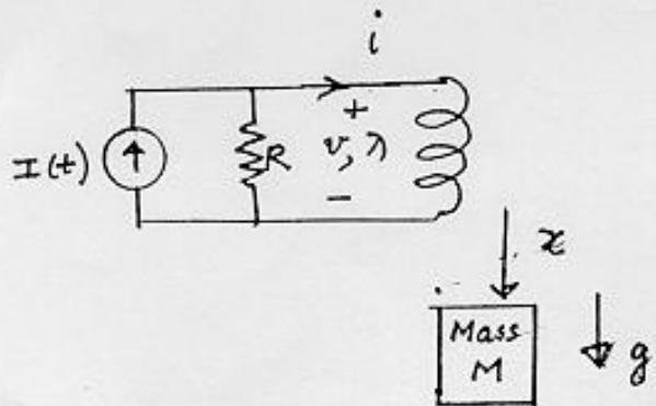
Distance  $x$  of the mass  $M$  is measured from a fixed reference.  $\lambda(i, x)$  is given as  $\lambda(i, x) = \frac{Ci^2}{x}$ .
