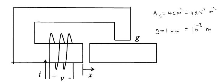
For the questions below, express all of these as functions of current (i) and/or position (x) and/or velocity and/or time as appropriate. You may neglect fringing in the gap, and you may assume the iron is infinitely permeable.
