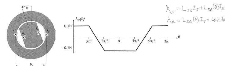
a) Plot the open circuit voltage (the case with stator current = 0) as a function of theta using the axes below. Label all points (compute all peaks). Do not use sinusoidal approximations.
