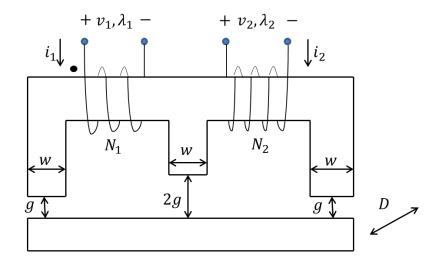
a) Given the dot marking for coil 1, finish the dot marking for coil 2 in the figure (5 points);
