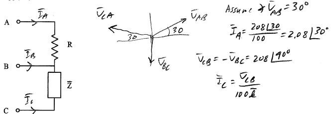
Resistor R is fixed at 100 Ohms. Impedance  $\overline{Z}$  is specified as a multiple  $\overline{k}$  R, where  $\overline{k}$  could be positive, negative, or even complex.
