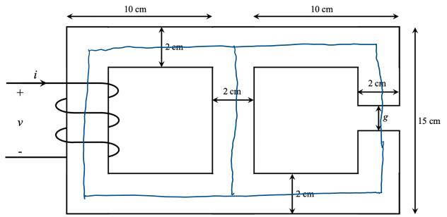
A coil is wrapped 300 times around an iron core with the given dimensions and a depth of 2 cm into the page. The iron has a permeability  $\mu = 2000\mu_0$  and contains an air gap of g=2 mm. Fringing effects can be neglected.
