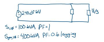
d) How much three-phase kVARs do we need to bring the combined power factor to unity? How would you connect the capacitors (in Wye or Delta) and why? (3 points)
