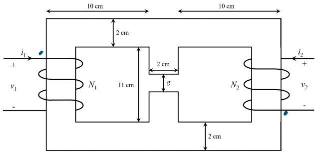
Two coils are wrapped around an iron core with the given dimensions and depth of 3 cm into the page. Coil 1 contains 400 turns and Coil 2 contains 200 turns. The iron has a permeability  $\mu$ =1500 $\mu$ <sub>0</sub> and contains an air gap of g=4 mm. Fringing effects can be neglected.
