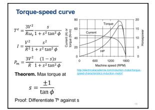
Torque-speed curve over a wider range  $Torque(Nm) \qquad Generating \qquad or generating \qquad or generative traking \qquad "re-generative traking"}$   $T^e = \frac{3V^2}{R\omega_s} \frac{s}{1+s^2 \tan^2 \phi}$ https://people.ucalgary.ca/~aknigh/electrical\_machines/induction/im\_trq\_speed.html
