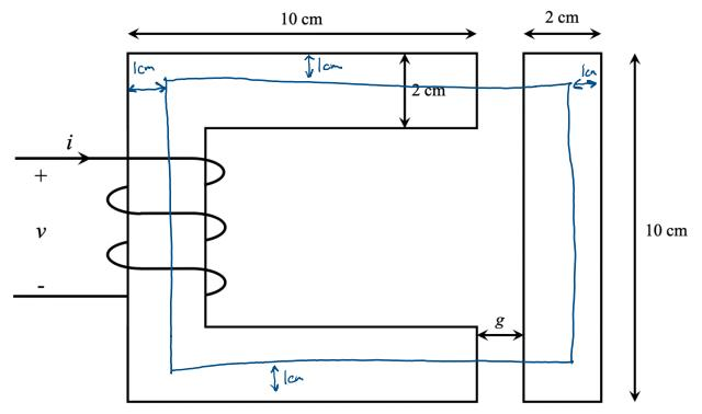
A coil is wound 150 times around an iron core (dimensions given above) with relative permeability 2500 that has an air gap g of 20 mm and depth into the page of 3 cm. With the voltage polarity and current direction as defined above:
