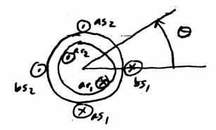
Write the  $3\times3$  inductance matrix for this machine in terms of  $L_s$ ,  $L_r$ , M and  $\theta$
