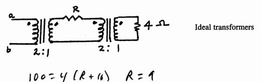
d) Write the two loop equations for the circuits shown
