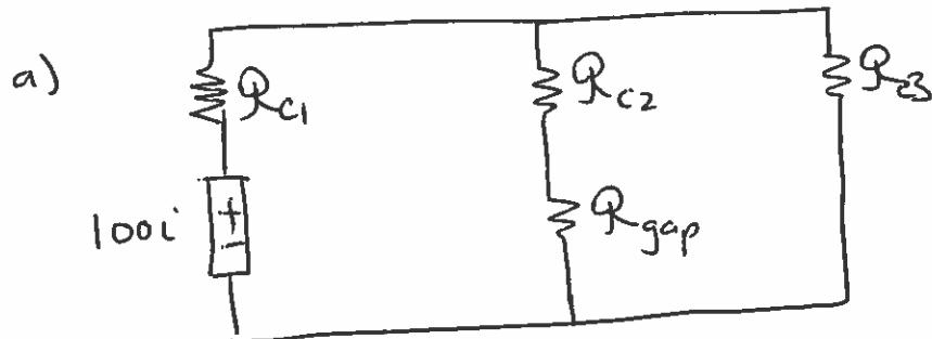
$$R_{C1} = R_{C3} = \frac{0.3}{1000\mu_0 \times 1 \times 10^{-4}} \\ = 2.387 \times 10^6 \text{ H}^{-1}$$
