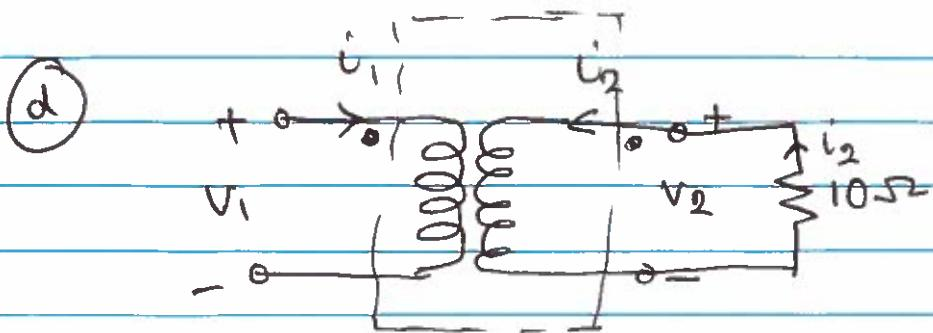
$$V_1 = L_1 \frac{di_1}{dt} + M \frac{di_2}{dt} \quad \text{--- (1)}$$
