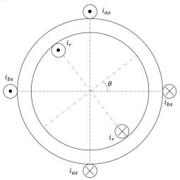
When the rotor's angular position is given by  $\theta$  as indicated, the flux linkages of the windings are given by:
