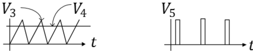
Figure 4: Comparison of the inputs and output of a voltage comparator circuit used for PWM control.
