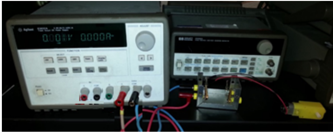
Figure 1: Circuit schematic and photo of the variable voltage source motor drive method.
