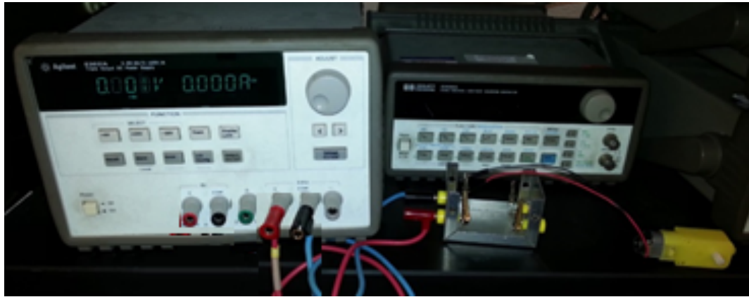
Figure 1: Circuit schematic and photo of the variable voltage source motor drive method.
