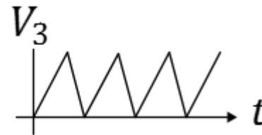
Figure 1: An amplifier with gain and offset controls will allow the designer to optimize the lowest and highest voltage of a periodic signal. For example, the waveform V_2 can be modified through an amplifier to resemble V_3 .
