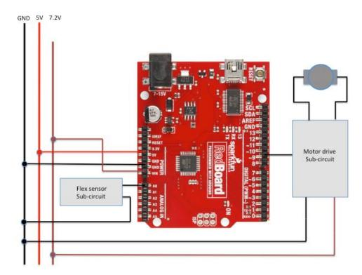
Now a program is needed to program the Arduino to emulate the wall-following circuit you put together in experiment 8. The following code illustrates how to connect 1 flex sensor to the Arduino and output a square wave with a duty cycle that changes as the flex sensor is flexed.
