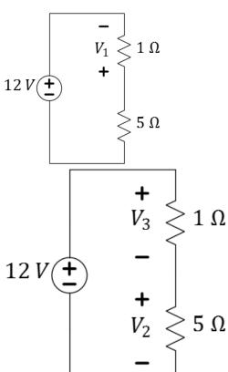
Step 2. Apply KVL to equate the sum of the voltage drops to the voltage being divided.
