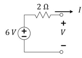
Step 1. Replace the voltage sources with short circuits and the current sources with open circuits.
