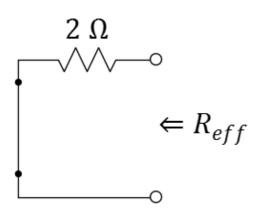
**Step 2.** Use series and parallel relationships between the remaining resistances to find  $R_{eff}$ .
