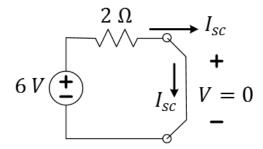
Step 2. Determine the current flow through the wire in the direction consistent with the arrow for *I*.
