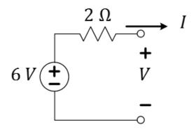
Step 1. Place a virtual short circuit (i.e. a wire) across the output terminal.
