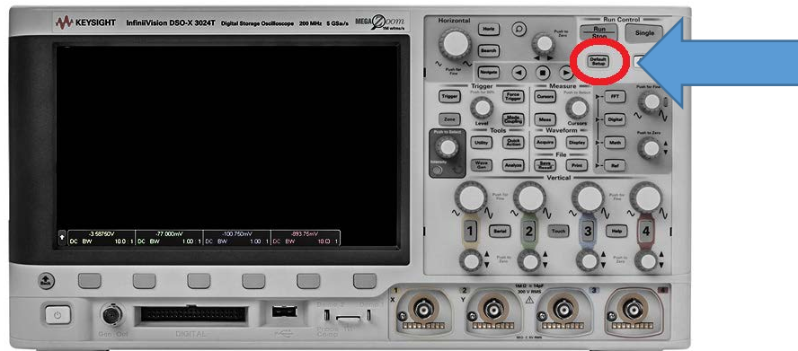
Figure 4: The oscilloscope's Default Setting.
