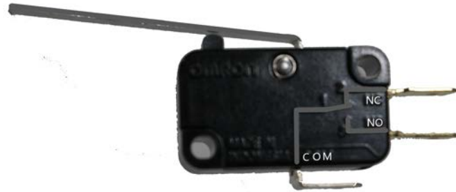
Figure 2: The snap-action (lever) switch. The second wire on the switch should be the “normally-open” ( NO ) connector which connects to the common ( COM ) when the switch is pressed. The other is “normally closed” ( NC ).
