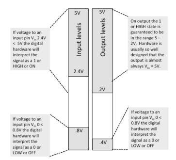
TTL LS family – this is the logic family that is used in our lab almost exclusively. The naming convention includes the designation of the type of TTL logic used. LS stands for Low power Schottky. It's advantage is lower power at the cost of speed. There are many other types of digital circuitry mostly optimized around speed, power, or device size.
