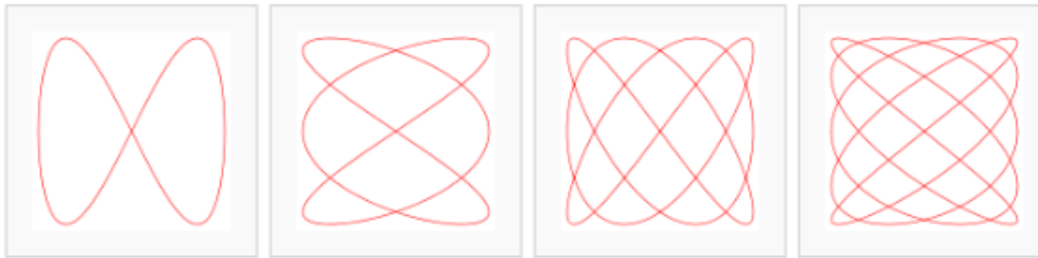
Figure 3: Typical Lissajous shapes. Source: http://en.wikipedia.org/wiki/Lissajous_curve . CC BY-SA 3.0.
