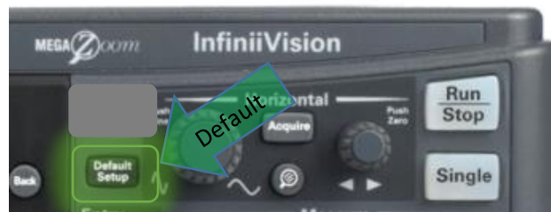
Figure 3: Always start by pressing the Default Setup on the oscilloscope.
