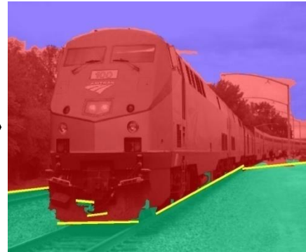
Fit Ground-Vertical Boundary with Line Segments
