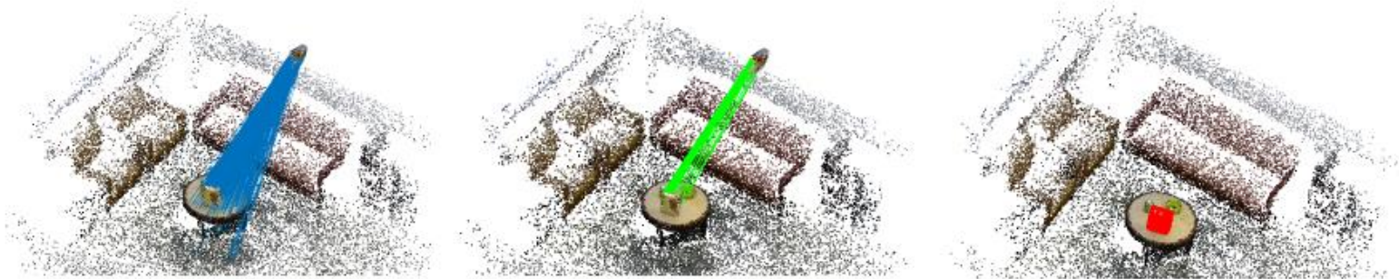
Fig. 8. Successful object pose estimation by TEASER on a real RGB-D dataset. Blue lines are the original FPFH [1] correspondences with outliers, green lines are the inlier correspondences computed by TEASER, and the final registered object is highlighted in red.
